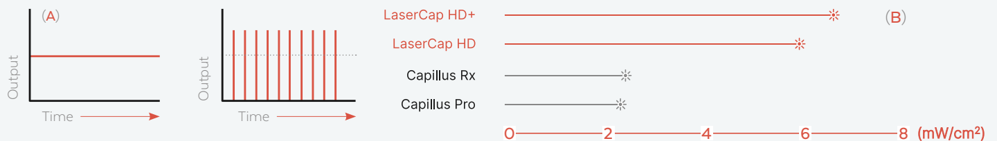
Figure 2: Higher peak intensity: Short, repetitive light pulses, illustrated in (A), allow for higher peak intensity output without excess generation of heat. As shown in (B), this allows LaserCap to deliver light at a much higher peak intensity compared to continuous output devices with similar power capabilities. As a result, photons can penetrate more deeply into tissues, delivering more energy to the base of the hair follicle.
